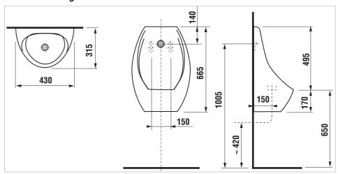
JIKA offers ceramic solutions geared towards the needs of businesses. One of them is Domino, an urinal with valve hole. Must be equipped with an external flushing valve (either pressure- or electromagnetic type). Complete product testing. 10-year warranty provided. Antibak prevents trapped dirt by having the inner ring and drains glazed. Sensor automatizes flushing.
